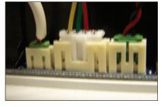
6. The fully seated connector is shown. It fits into the socket only one way.
