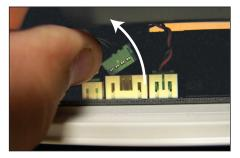
3. Unplug the connector (if needed, pry it up with a small tool). Tape the connector and its cable away from any moving parts.
