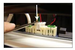
5. Plug the 4-pin connector into the socket. Press it into place with a small tool. Position the cable away from any moving parts.
