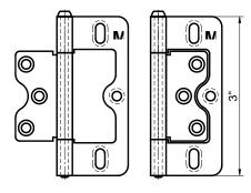
For Deco Frames, L Frames, Z Frames and Hang Strip (OM) 3" Offset Rabbet Hinge (M)
