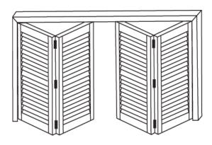
The max frame to frame measurement should be from floor to the top of fascia.
